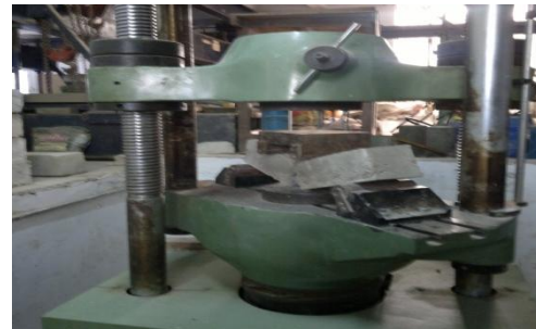
Fig – 2 Beam after Flexural Test
