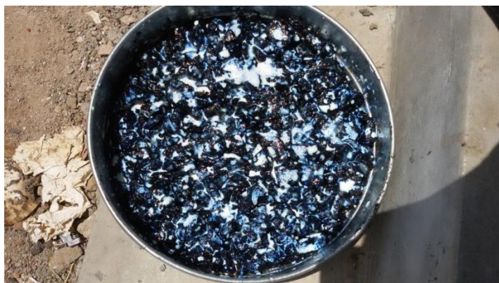
Fig -2 Mould with Epoxy and Geo-sheet
