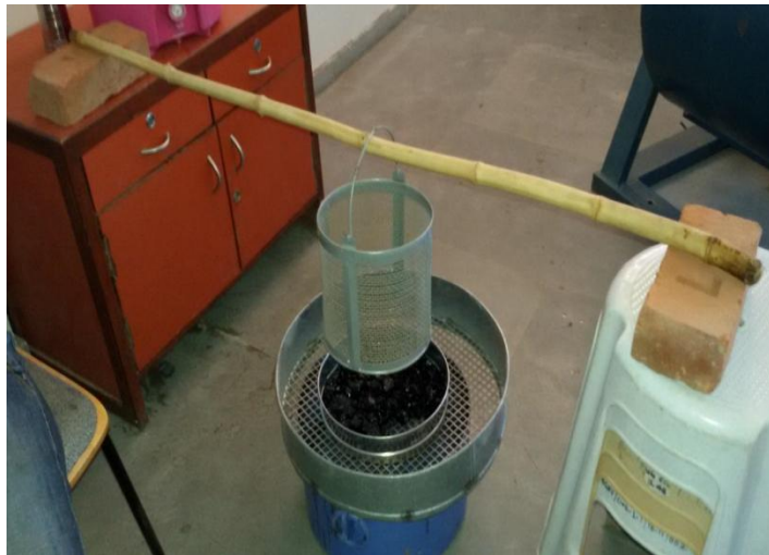
Fig – 3 Sprinkler method arrangements
