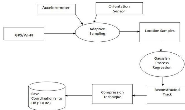
Fig. 2 Data Flow Diagram / Work flow Diagram
