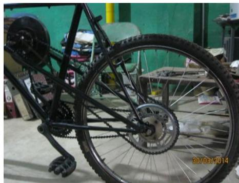
Two clutches are used during the process. 1st one is used to slow down the rear wheel by engaging it with the flywheel and stores the kinetic energy in that flywheel. 2nd is used to regain the acceleration by engaging it to retrieve the energy from the flywheel.
