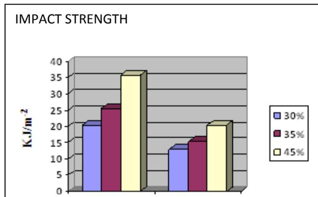
**Fig 4 Impact strength of untreated and treated sisal fiber**
