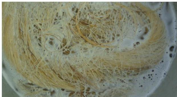
Fig 1 Soaking of Sisal fiber in NaOH
