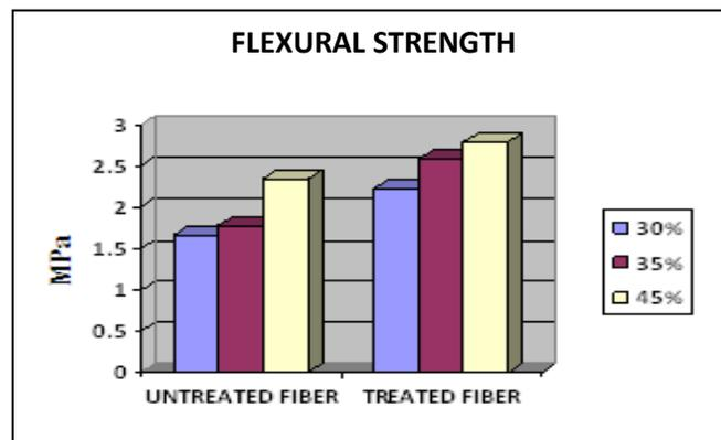
Fig 3 flexural strength of untreated and treated sisal fiber
