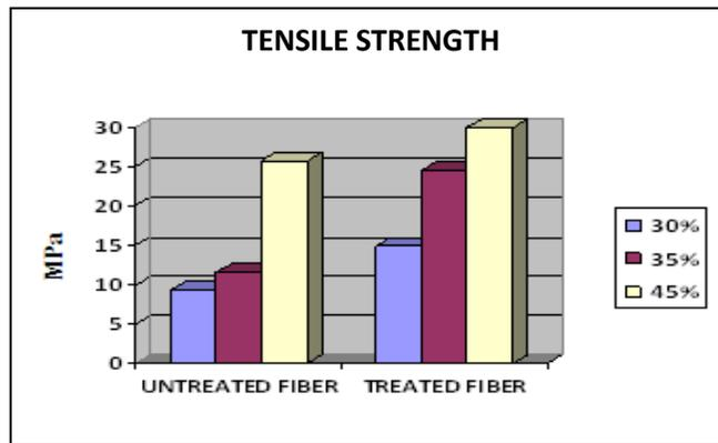
Fig 2 Tensile strength of untreated and treated sisal fiber
