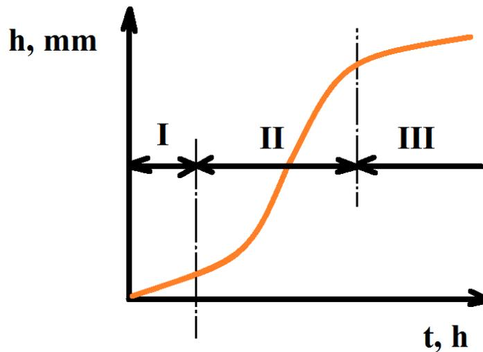
**Fig.1 Average depth of erosive wear depending on operating time of blades**
