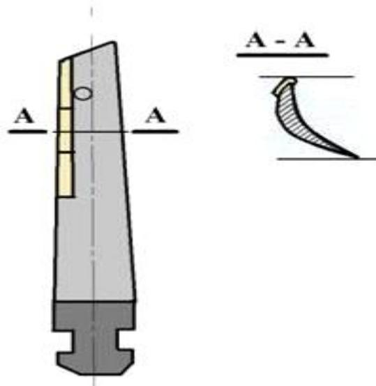
Fig.3 Moving blade with stellite cover plate
