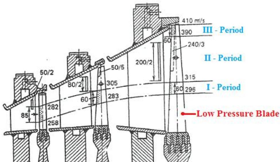
Fig. 2 The steam path of steam turbine with slits in the exit portions of nozzle blades (figures indicate the size of slits, mm, and circumferential velocity of blades, m/s).
