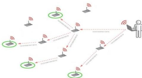
Fig 1. Over The Air Programming
