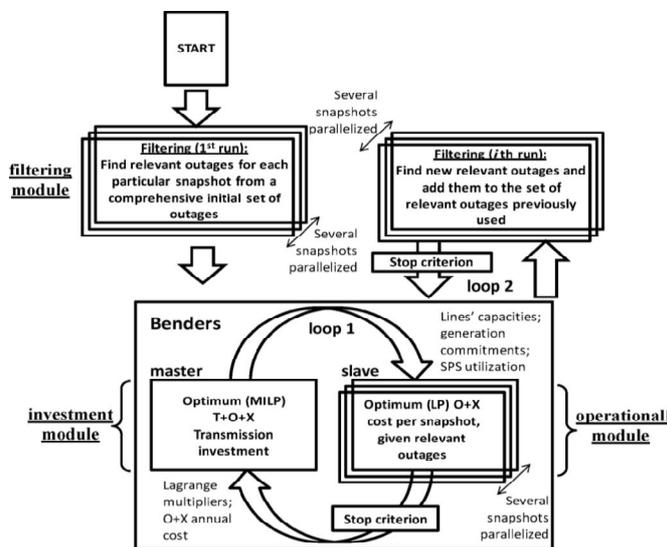
Figure.1 General Bender algorithm with 3 modules
