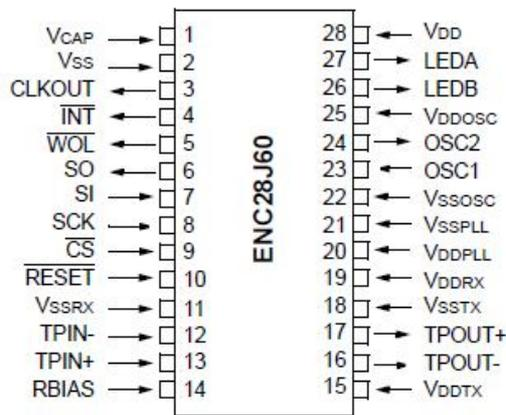
**Figure 3 Pin diagram of ENC 28J60**
