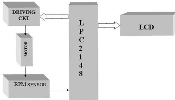
**Figure 2 RPM Interfacing.**
