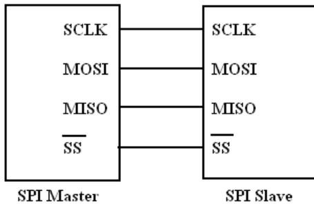
Figure 4 SPI Interface
