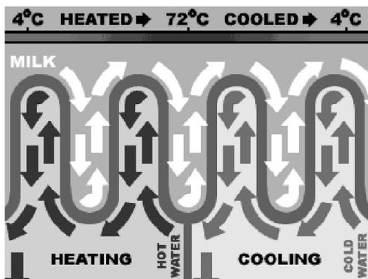
*Figure 1 Pasteurization process.*
