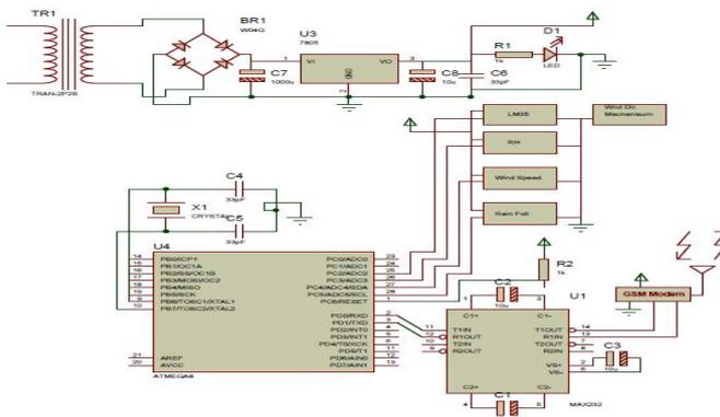
Fig 7: Transmitter Circuit Schematic
