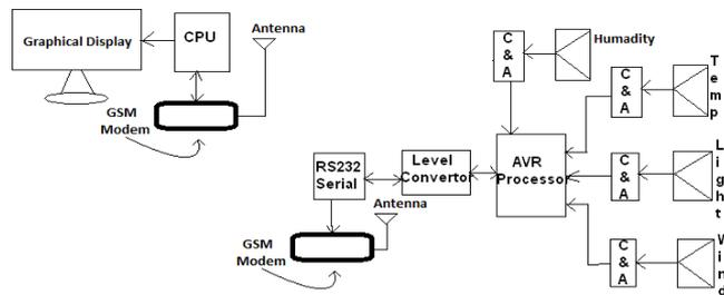
Fig. 4 Block diagram for transmitter and receiver.
