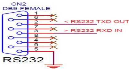
Fig 6 RS 232 pin configuration
