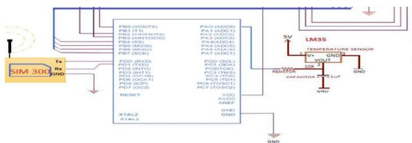
Fig: 10 interfacing of LM 35 with controller(sample for temperature)
