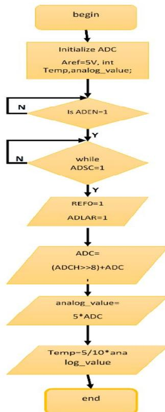
Fig 11: Flowchart for ADC conversion
