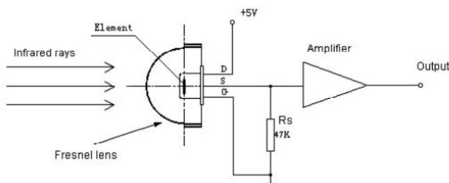
Fig. 6 Human Body Detection using PIR Sensor[3]
