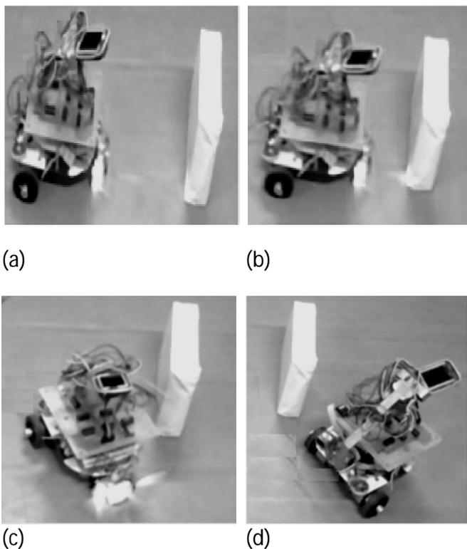
Fig. 8(a) to (d): Maneuvering of prototype robot across non-human obstacle
