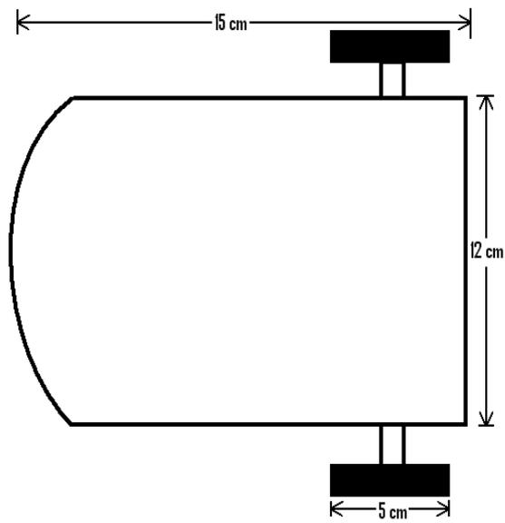
Fig. 2 Chassis Dimensions
