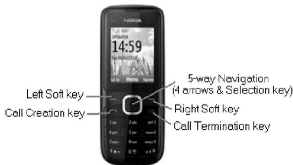
Fig. 10(a): Nokia C1-10 Model with control keys
