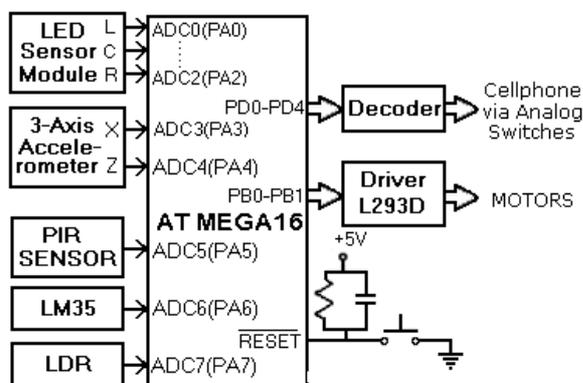
Fig. 7 Microcontroller System Interfacing
