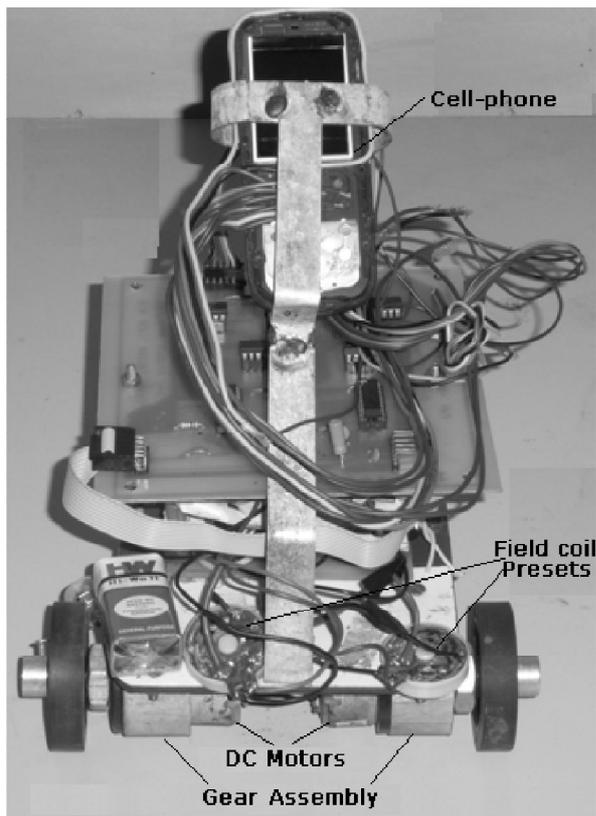
Fig. 3 Backend view of Robot Prototype
