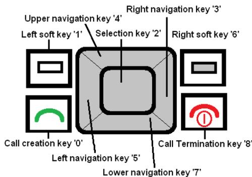
Fig. 10(b): Nokia Model C1-01 control keys with assigned codes
