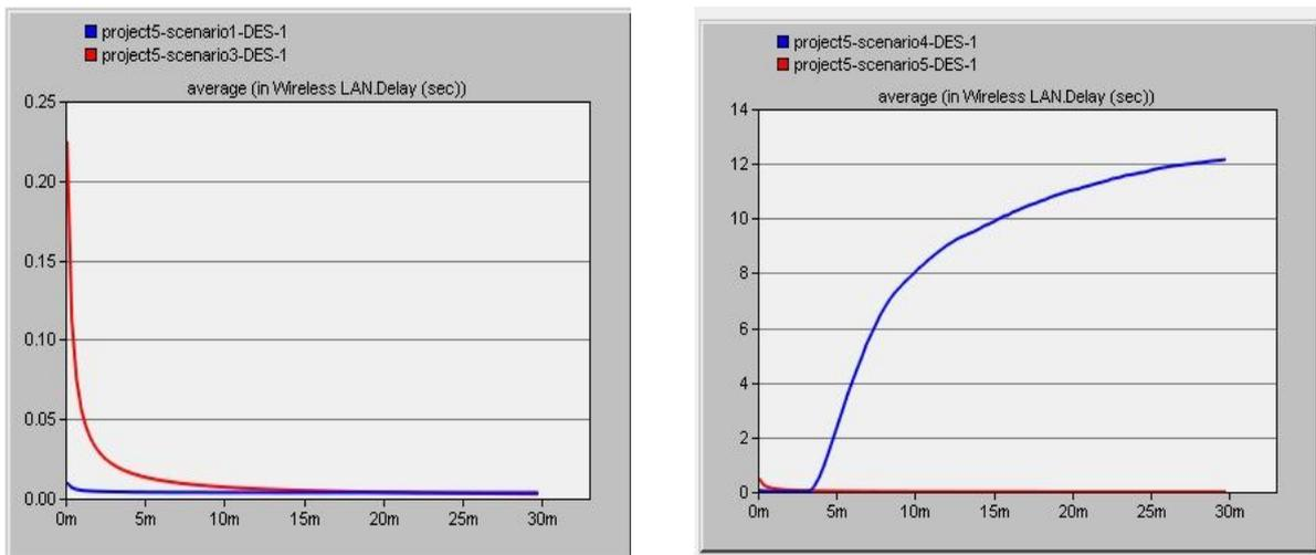
Figure2 Wireless LAN Delay (sec)
