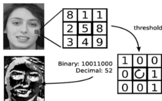
Fig. 5 The LBP operator thresholds each pixel against its neighboring pixels and interprets the result as a binary number. In the bottom image each gray-level value corresponds to a different local binary pattern.
