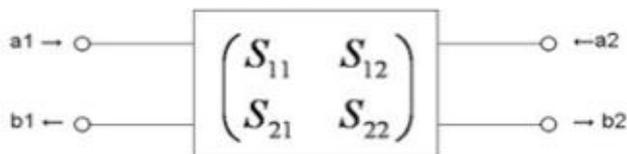
Figure 4: S Parameter Two Port Model
