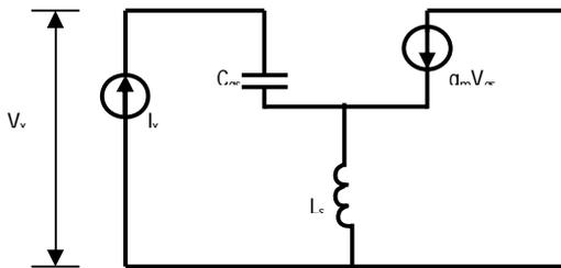
Fig. 3-1 Small signal model
