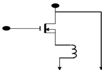
Fig.3 Inductive source degeneration
