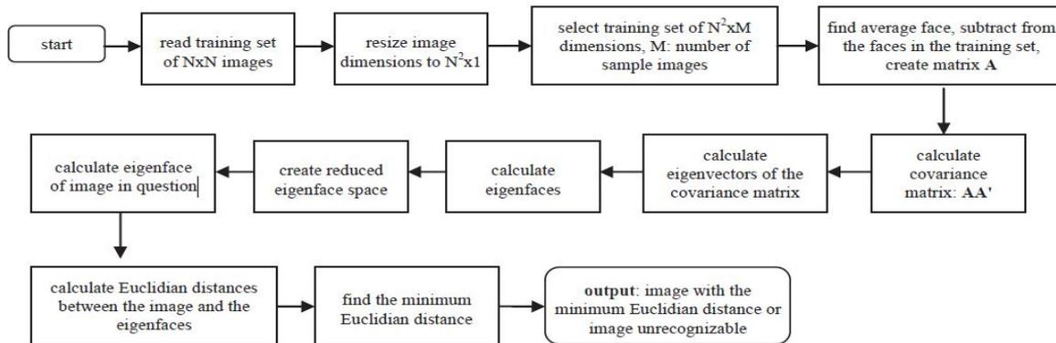
Fig 1. Flowchart of the algorithm of the Eigen faces method
