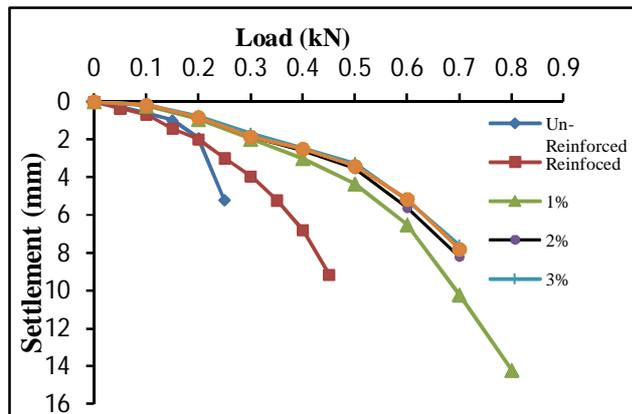
Figure 6: Load intensity versus normalized settlement curves at reinforcement depth B/4 with Biaxial prestressing force of different magnitude.
