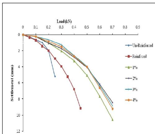
Figure 4: Load intensity versus normalized settlement curves at reinforcement depth B/4 with Uniaxial prestressing force of different magnitude.
