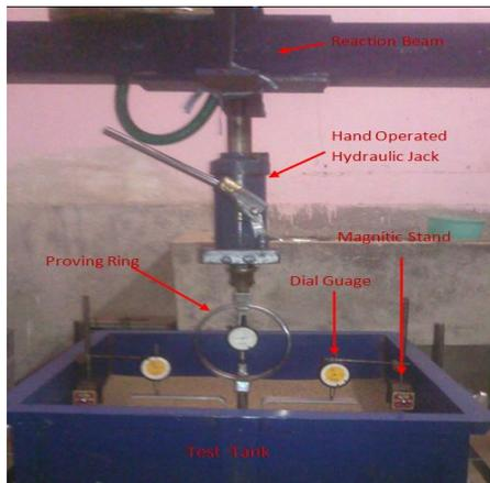
(b) Actual Laboratory Plate load Test Tank
