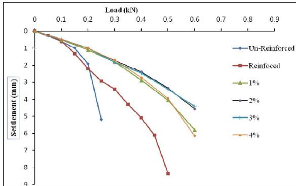
Figure 3: Load intensity versus normalized settlement curves at reinforcement depth B/2 with Uniaxial prestressing force of different magnitude.
