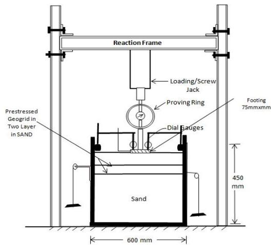
(a) Elevation of Laboratory Test Tank
