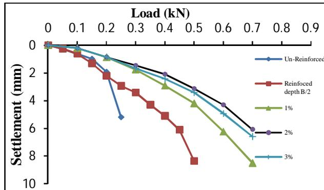
Figure 5: Load intensity versus normalized settlement curves at reinforcement depth B/2 with Biaxial prestressing force of different magnitude.
