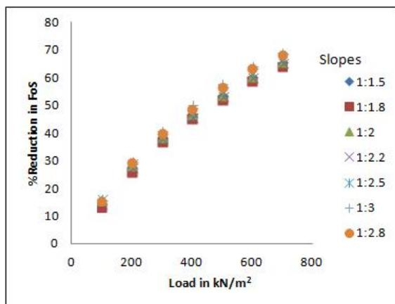
Figure 5: % Reduction in Factor of Safety
