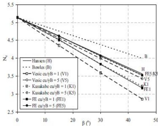
Figure 1:  $N_c$  with slope angle and normalized sloped height.
