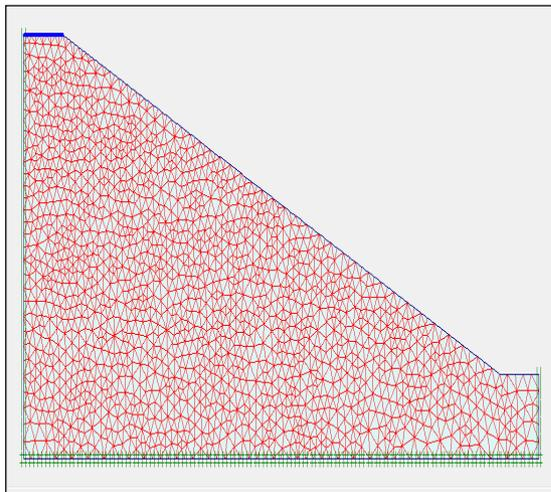
Figure 3: Formation of mesh in Plaxis 2D software
