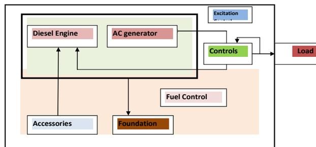
Block dia: Subsystems of PSS acoustic container
