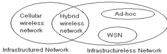
**Fig1: Classification of Wireless Sensor Network**
