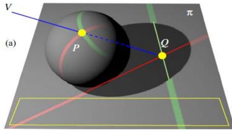
**Figure 1. Illustration of the principle and details of geometric shadow scanning. Point Q is the point on the reference plane that lies behind point P along ray V**
