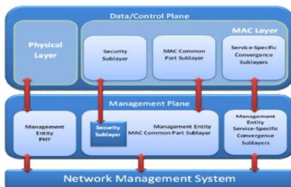
Figure 1. WiMAX Protocol Layers
