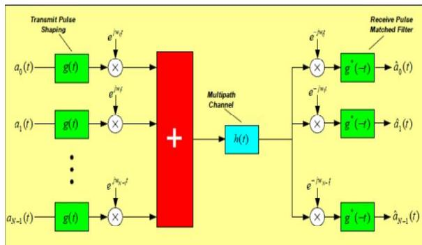
**Figure 2: Basic Architecture of an OFDM System**
