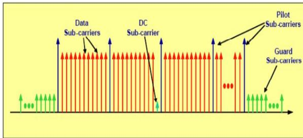
**Figure. 3: OFDM Sub-carrier Structure**
