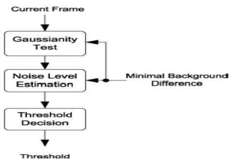
Fig.2. Block diagram of threshold determination algorithm
