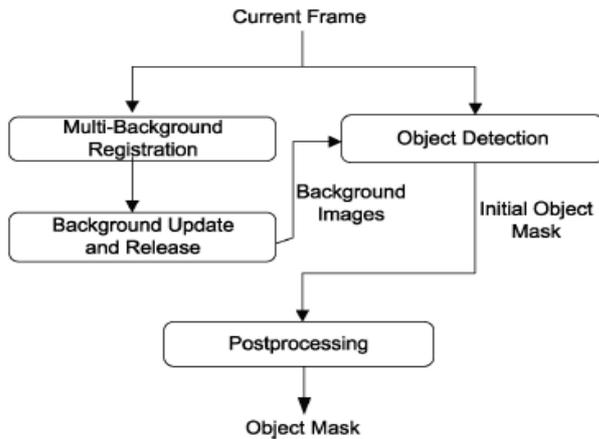
Fig. 1. Block diagram of the video segmentation algorithm.
