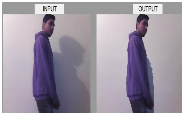
**Fig. Proposed Background Subtraction and Shadow Removal Algorithm**
