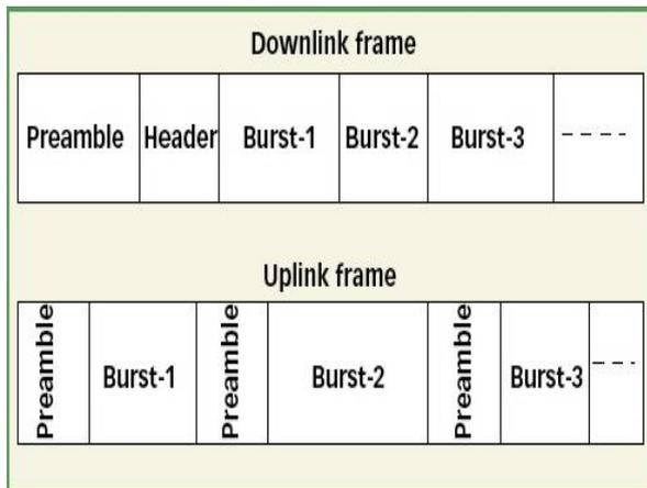
1. Typical downlink (top) and uplink (bottom) frame formats are represented here.
