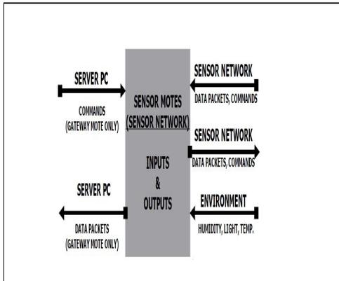
**Figure 5: Sensor Mote Component I/O**
