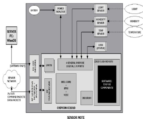
**Figure 6: Sensor Mote Block Diagram**
