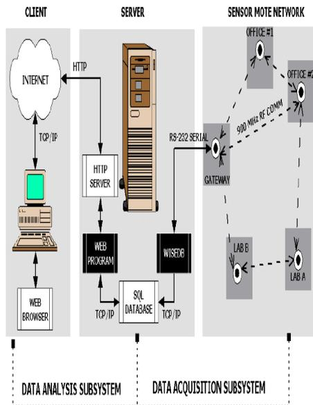
**Figure 1: WISNET System Block Diagram**
