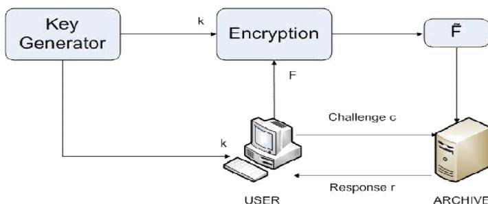
Fig.1.Schematic view of a proof of retrievability based on inserting random sentinels in the data file network resources. Furthermore, the I/O to establish the data proof interferes with the on-demand bandwidth of the server used for normal storage and retrieving purpose. The problem is further complicated by the fact that the owner of the data may be a small device, like a PDA
