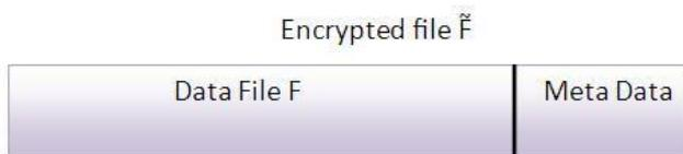
Fig. 4. The encrypted file  $F_e$  which will be stored in the cloud specifying the block number  $i$  and a bit number  $j$  generated by using the function  $g$  which only the verifier knows. The verifier also specifies the position at which the meta data corresponding the block  $i$  is appended. This meta data will be a  $k$ -bit number. Hence the cloud storage server is required to send  $k+1$  bits for verification by the client.
