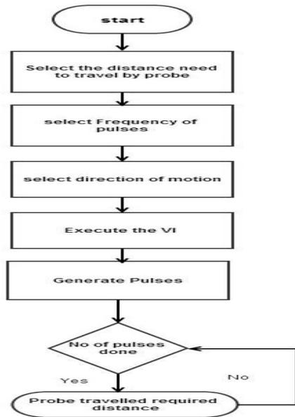
Figure 7 Flowchart for linear motion of probe
