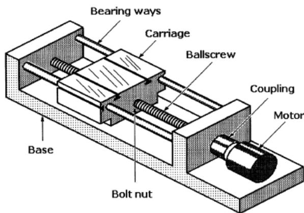
Figure 2. Ball screw slide mechanism
