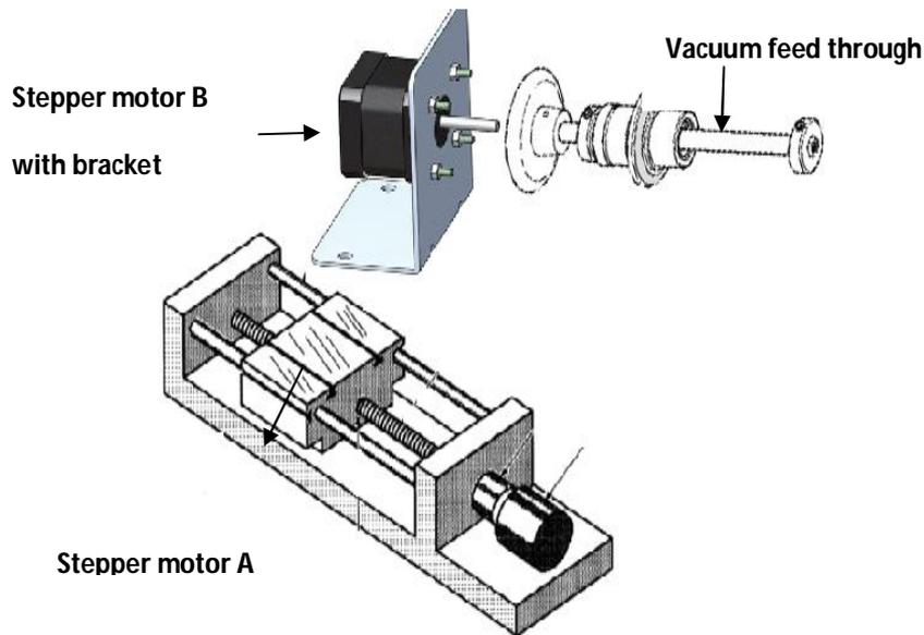
Figure 5 Feed through couple with orthogonal bracket for radial motion.
