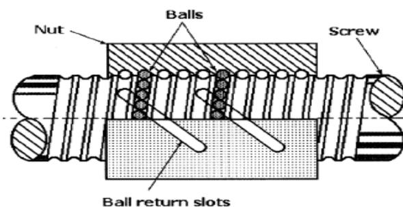
Figure 1. Ball screw drive.
