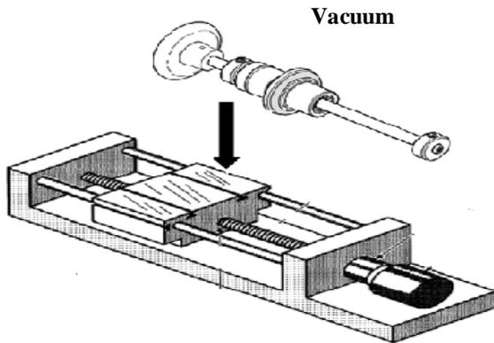
Figure 3. Vacuum feed through placed on carriage of linear slider.
