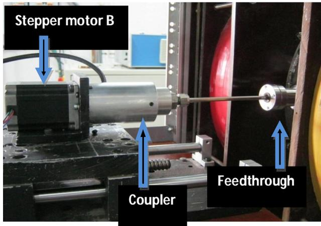
Figure 6 For rotational motion Stepper motor B coupled with feed through
