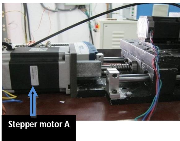
Figure 4 For linear motion stepper motor A coupled with ball screw
