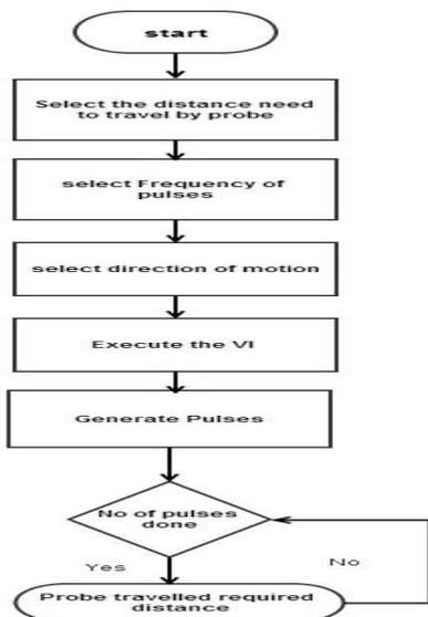
Figure 8 Flowchart for angular motion
