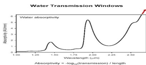
Figure 1: Water Absorbance spectra
