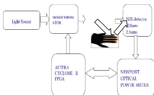
**Figure 3:** Digital spectrophotometer
