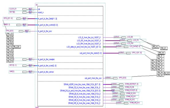
Figure 6: Full soft core system for glucose analysis.
