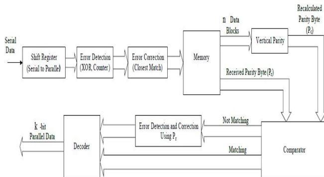
Fig.4. Block diagram of the receiver.
