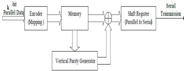
Fig.3. Block diagram of the transmitter.
