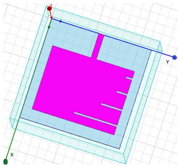
Fig.1 Strip line fed rectangular patch antenna
