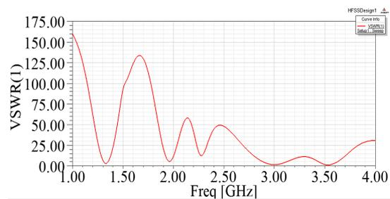
Fig.12 VSWR curve of probe fed antenna
