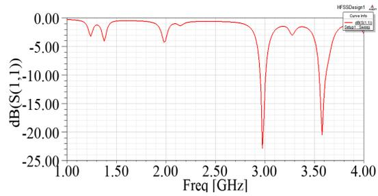
Fig.5 S parameter Vs frequency plot of inset fed antenna
