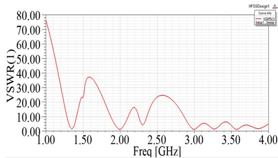
Fig.3 VSWR curve of strip line fed antenna
