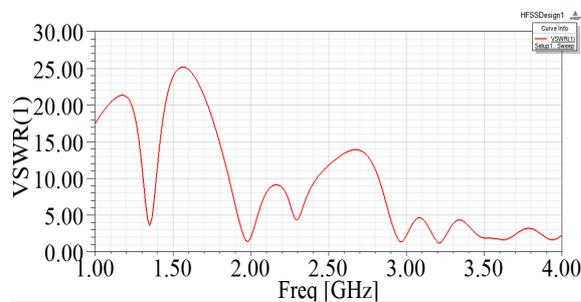
Fig.9 VSWR curve of edge fed antenna
