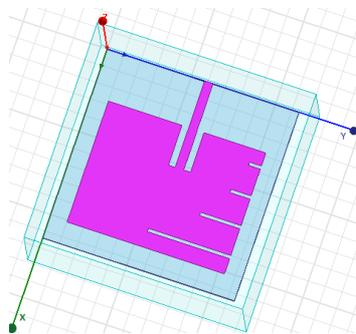
Fig.4 Inset fed rectangular patch antenna
