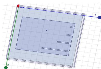
Fig.10 Coaxial probe fed rectangular patch antenna
