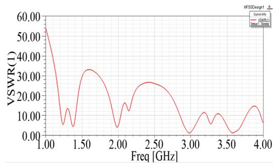
Fig.6 VSWR curve of inset fed antenna
