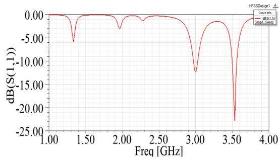
Fig.11 S parameter Vs frequency plot of probe fed antenna
