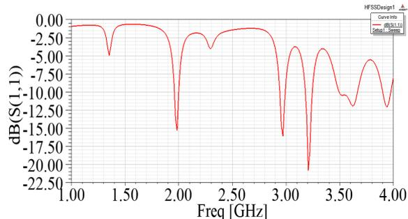
Fig.8 S parameter Vs frequency plot of edge fed antenna
