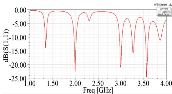
Fig.2 S parameter Vs frequency plot of strip line fed antenna
