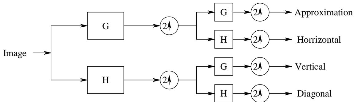
Figure 3.2 Undecimated Wavelet Transform - one level decomposition
