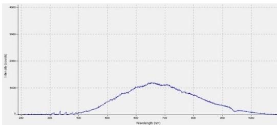
Fig. 6: Continuum spectrum obtained because of air breakdown
