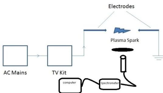
Fig.5: Experimental set up for recording the optical spectrum of electric spark.
