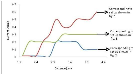
Fig. 6: Distance between electrodes Verses Breakdown current for the set ups shown in fig. 2, 3 and 4.
