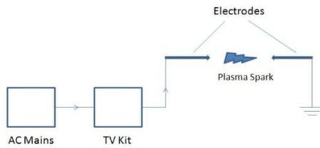
Fig 1:- Experimental set up for plasma spark gap
