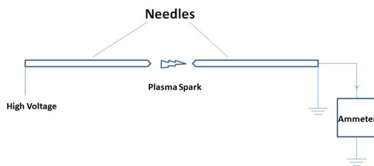
Fig.2: Breakdown current measurement between two pointed needles.
