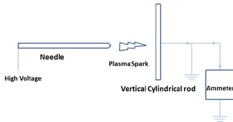
Fig.4: Breakdown current measurement between one pointed needles and vertically kept steel rod having diameter of 9.5 mm.
