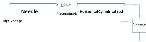
Fig. 3: Breakdown current measurement between one pointed needles and steel rod having diameter of 9.5 mm.
