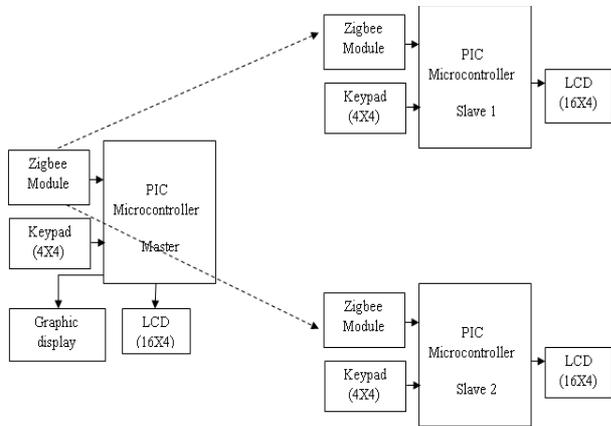
**Figure 1.7 Block Diagram of Navigation system to assist visitors**
