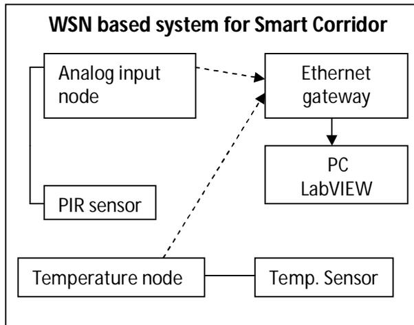
**Figure 1.3 Block diagram of WSN based system for Smart Corridor**
