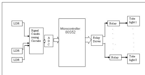
**Figure 1.2 Block Diagram of developed lighting Control System [12]**
