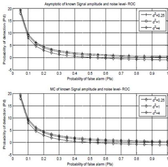
Figure.3: Probability of Detection Vs Probability of False Alarm
