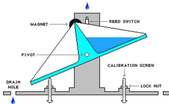
Figure 2. Working of TBRG
