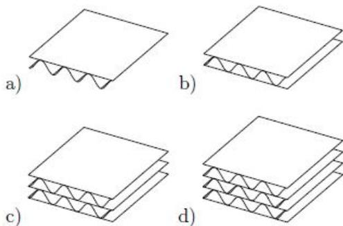
Figure 2.1 Types of corrugated board a) Single face b) Single wall c) Double wall. d) Triple wall.
