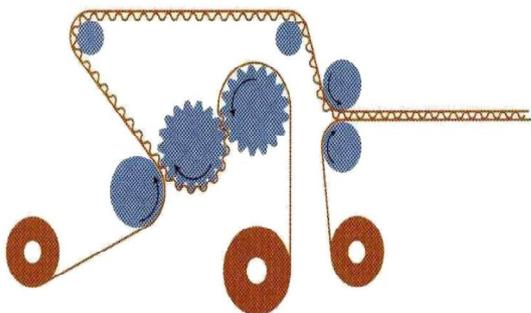
Figure 2.2: The manufacturing of a single wall corrugated board.
