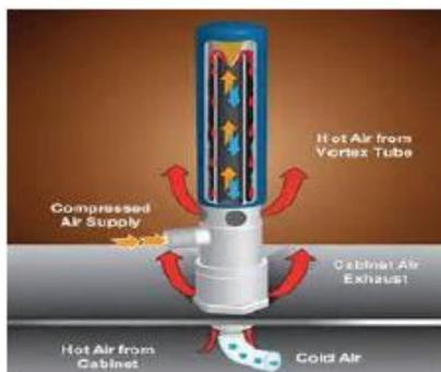
Fig: 8) MECHANISM OF RANQUE EFFECT
