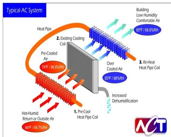
**Step 1.** Incoming return or outside 84°F air is pre-cooled to 74°F DB/ 96.8%RH by the pre-cool heat pipe coil.
