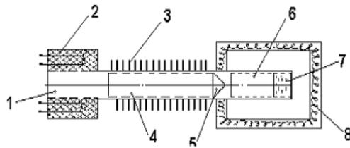
Fig. Sorption heat pipe. Longitudinal cross section, [3]. (1) Vapour channel;(2) porous sorption structure(3),finned surface of heat pipe evaporator/condenser;(4) porous wick inside heat pipe;(5) porous valve;(6) heat pipe low temperature evaporator with porous wick;(7) working fluid accumulated inside the evaporator; and (8) cold box with thermal insulation.
