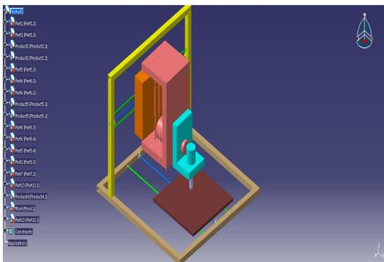
Fig.2.1 Proposed model of angular drilling machine
