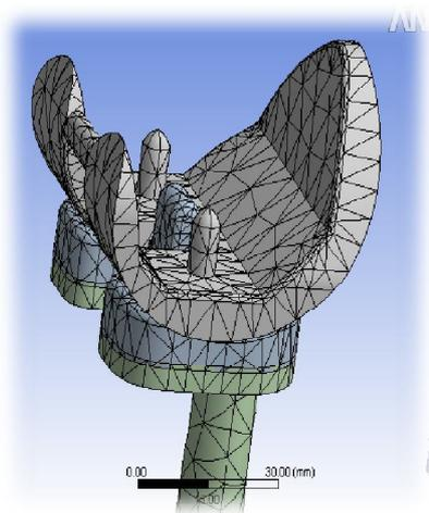
Fig.6. Meshing model of Knee Implant
