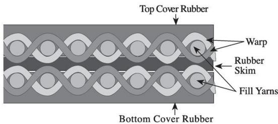
**Fig. Conveyor belt construction**
