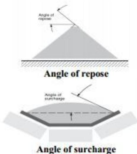
**Angle of surcharge  $\beta$ :** The area of the section "S" may be calculated geometrically adding the area of a circle A1 to that of the trapezoid A2. The value of the conveyed volume  $Ivt$  may be easily calculated using the formula:
