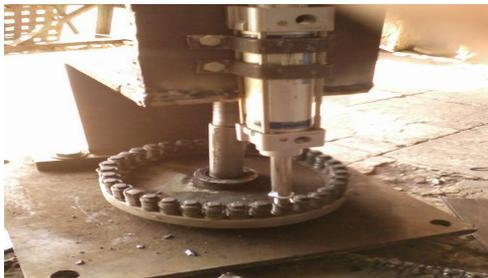
After all that, take a pneumatic cylinder of pressure 10 bar fitted on plate of body. To punch a latter on metal.
