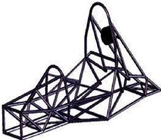
Fig-3: Space frame chassis
