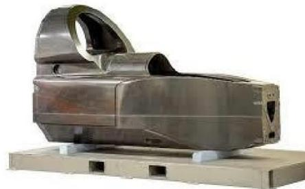
Fig-4: monocoque chassis
