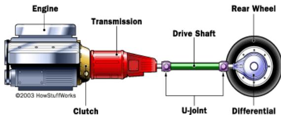
**1) Manual transmission:** Manual transmission was the first invented transmission system. the driver needs to disengage the clutch to disconnect the power from the engine, first select the target gear and engage the clutch again to perform the gear change again. It always need some time to acquire the skills for new driver.
