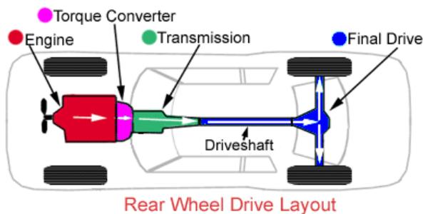
Fig. General power transmission system
