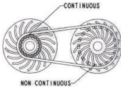
Figure (3) – Variable Diameter Belt CVT
