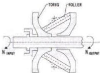
Figure (2) – Toroidal CVT
