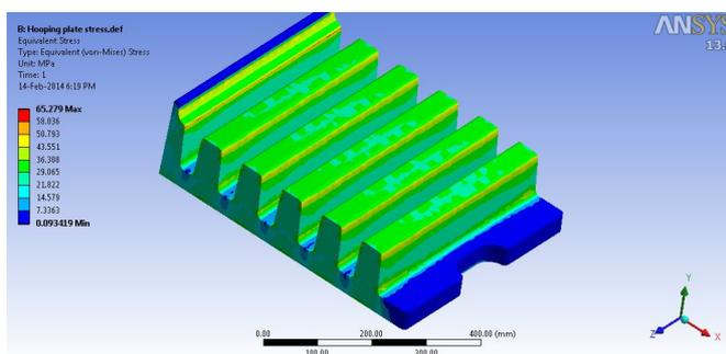
Figure 4: Von mises stress
