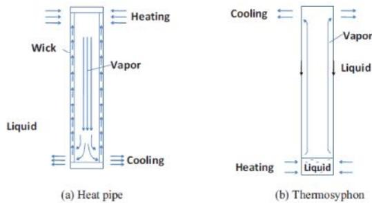
**Figure 1: Two-Phase Closed Thermosyphon and Heat Pipe** <sup>[9]</sup>
