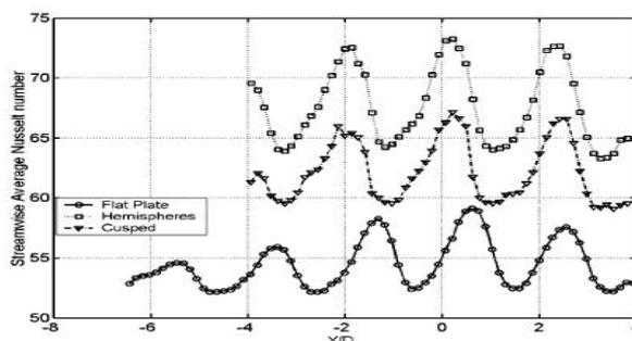
Fig.5 : Nusselt number variation with Flat, Hemispherical and Cusped shape dimple plate at  $H/D=4$ .
