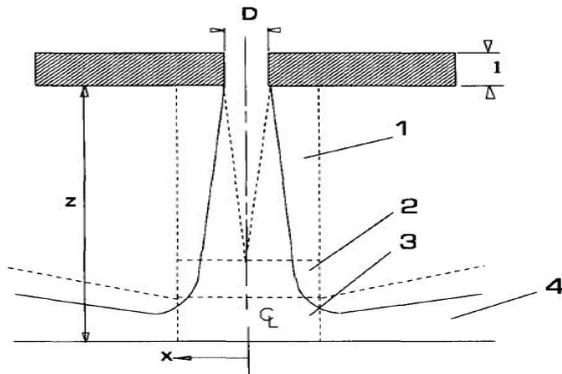
Figure 1 Flow zones in an impinging jet. Zone 1, initial mixing region; zone 2, established jet; zone 3, deflection zone; zone 4, wall jet
