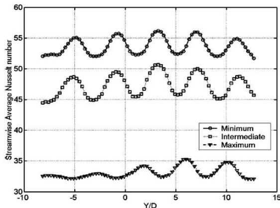
Fig.2: Nusselt number distribution with different flow schemes.
