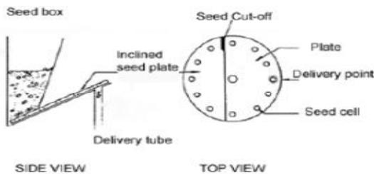
Fig:-inclined type seed meter
