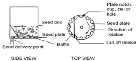
Fig 3. Horizontal plate type meter
