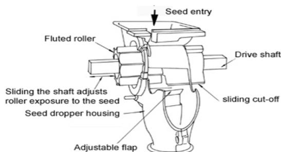
**Figure 2. The general form of the fluted roller type of external force feed seed meters**
