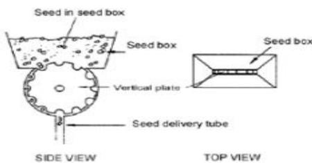
Fig:-vertical plate type seed meter
