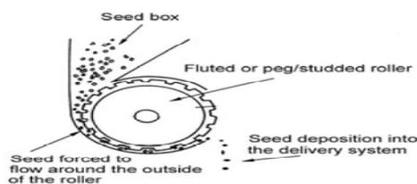
**Figure1: General principle of operation of 'external force feed' seed meter types**
