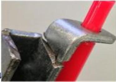
Pic 2: Typical Bracket failure
