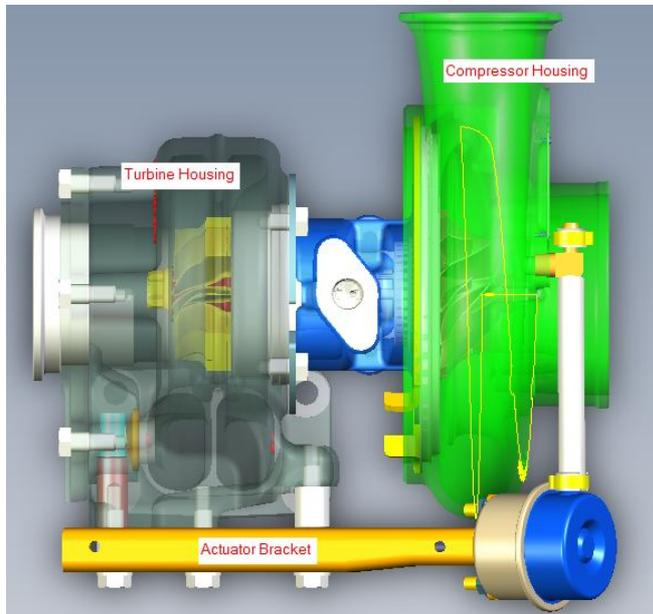
Pic1: Actuator Mounted on Turbine
