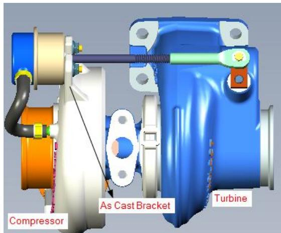
Pic 4: As Cast Mounting for Actuator
