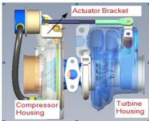
Pic 3: Compressor Mounted Actuator
