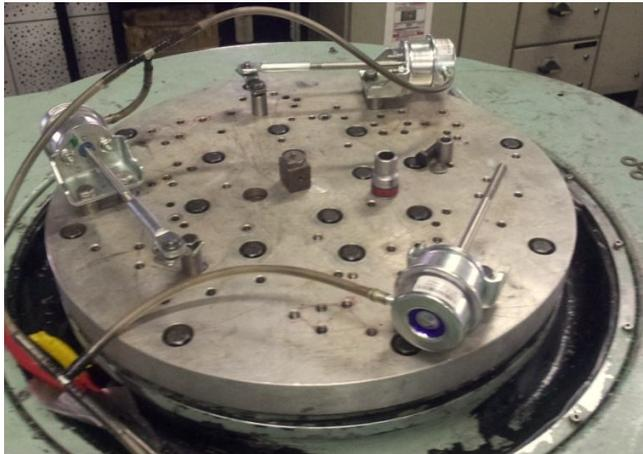
Pic 10: Typical Shaker Rig Test Set up for Sheet Metal Actuator Bracket
