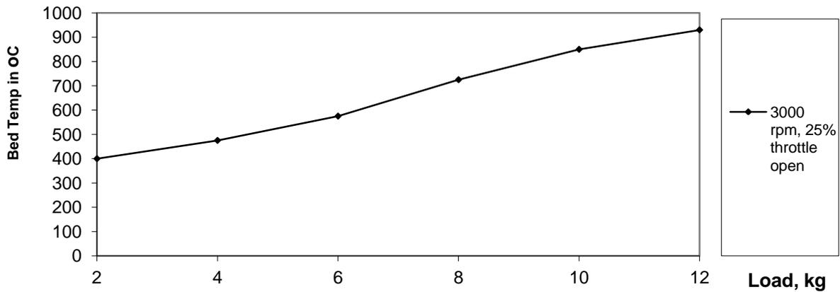
Fig. 6 Load Vs. Bed Temperature
