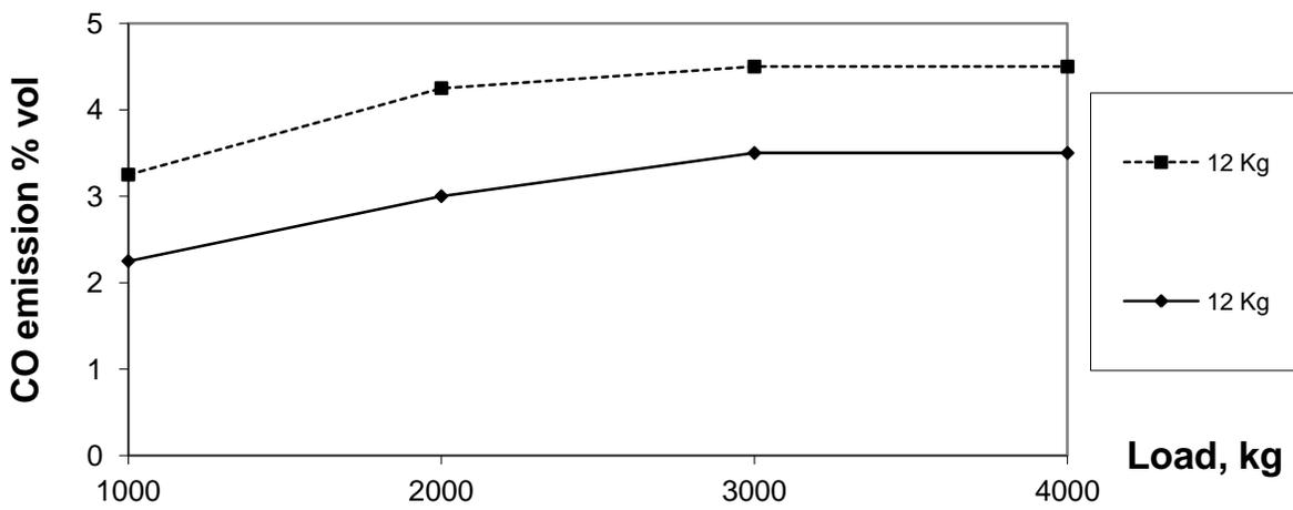
Fig 10. Load vs. CO emission %vol
