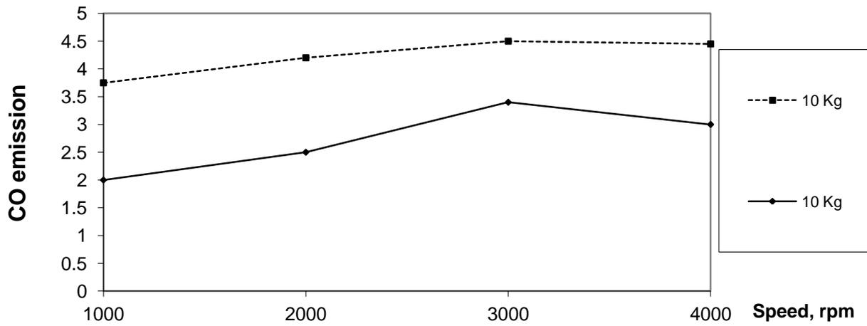
Fig 9. Speed vs. CO emission
