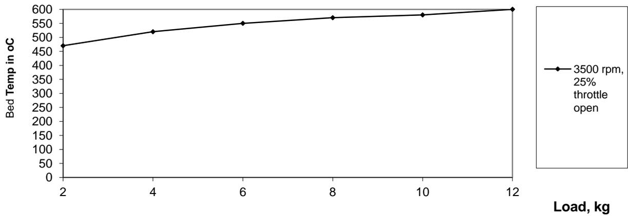
Fig. 7 Load Vs. Bed Temperature
